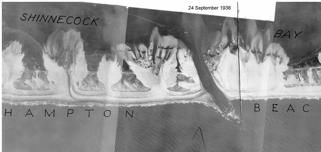
Figure IV-3-26. Shinnecock Inlet, Long Island, New York, 24 September 1938. Taken three days after Great New England Hurricane breached the barrier, this image shows the new Shinnecock Inlet and many overwash fans along the adjacent shore. Immediately after the storm, all the inlets along this stretch of the coast trended left of the shore-perpendicular. (Photograph mosaic from Beach Erosion Board archives)
